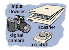
are other devices similar to a mouse that can be used in its place. A **trackball** has the ball on top and you move it with your finger. A **touchpad** allows you to move your finger across a pressure sensitive pad and press to click.
